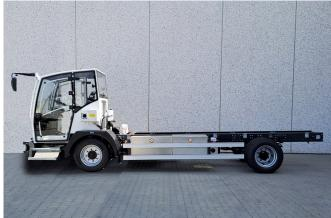
Vestergaard Company's fully electric chassis is able to carry a number of applications, e.g. water and lavatory carts or de-icing units. The smallest version is equipped with a 40 kWh lithium-ion battery with enough capacity to drive up to approximately 50 km and operate for approximately 12 hours. Also available with 60 or 70 kWh battery.
