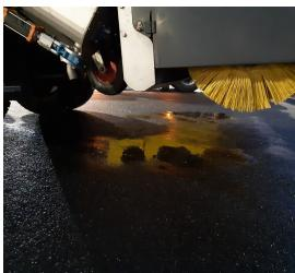
Vestergaard Company's Glycol Recovery Vehicle (GRV) has been developed to handle the important task of minimizing environmental impact of spent deicing fluid
